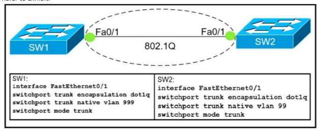
Which action do the switches take on the trunk link?
