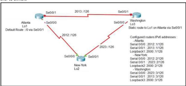
An engineer is configuring the NEW York router to reach the Lo1 interface of the Atlanta router using interface Se0/0/0 as the primary path. Which two commands must be configured on the New York router
